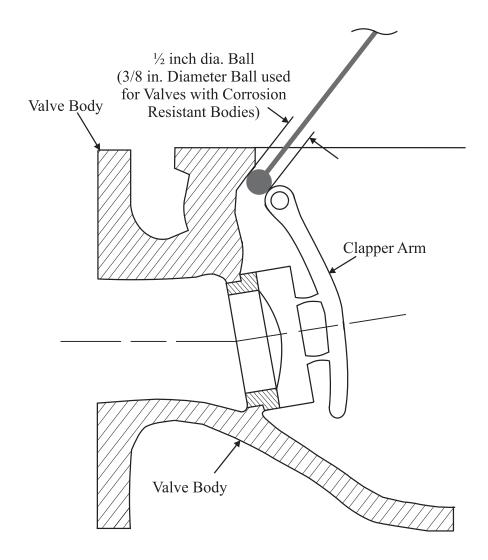
Figure C-2. Hub of the Clapper Arm and Inside of the Body Clearances
