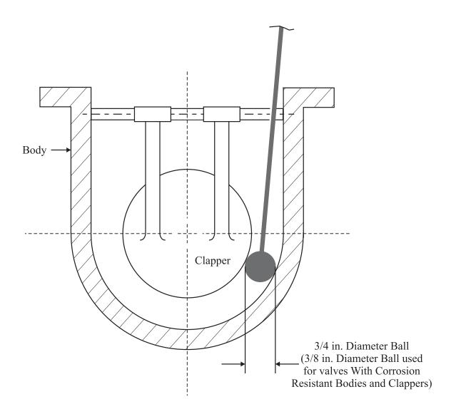
Figure C-1. Periphery of the Clapper and the Inside of the Body Clearances
