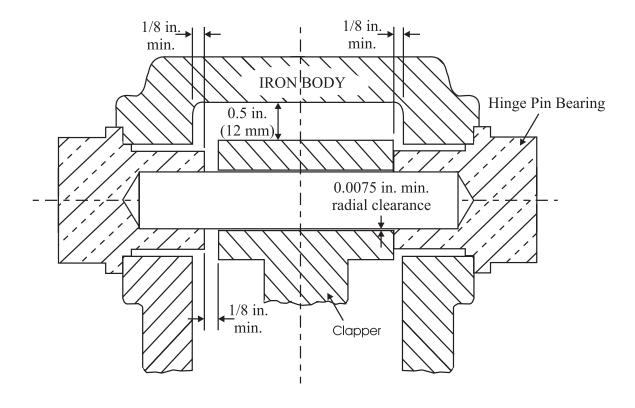
Figure C-3. Hinge Pin Clearances
