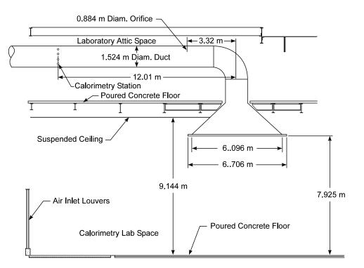
Figure C-1 Diagram of the 5 MW Fire Products Collector
