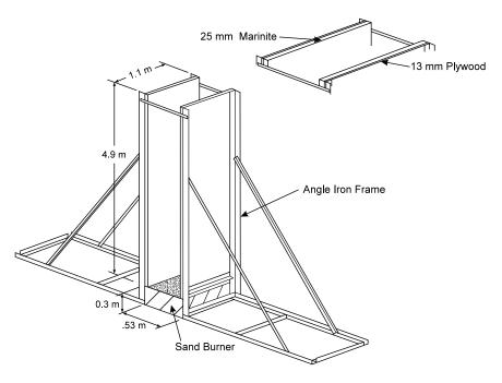
Figure C-2 Schematic of Parallel Panel Test Apparatus
