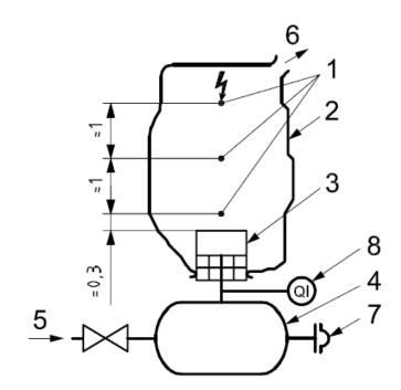
Key 1 ignition sources 2 plastic bag ( $\emptyset \ge 1.2 \text{ m}$ ; length  $\ge 2.5 \text{ m}$ ; foil thickness  $\ge 0.05 \text{ mm}$ ) 3 flame arrester 4 explosion-pressure-resistant containment (vessel or closed pipe work) 5 mixture inlet with shut-off valve 6 mixture outlet 7 bursting diaphragm 8 flame detector for indication Dimensions in meters
