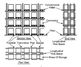
Fig. 1 Typical Double-Row (Back-To-Back) Rack Arrangement
