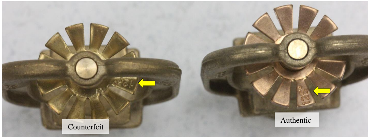
Figure 2. Authentic Tyco nozzle (right) and counterfeit (left). Both deflectors are stamped with the nominal spray angle. The authentic deflector appears to be a different material and is a different color than the counterfeit.
