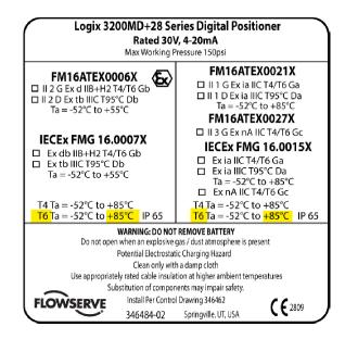
Figure 1 – Incorrect Nameplate, with error highlighted
