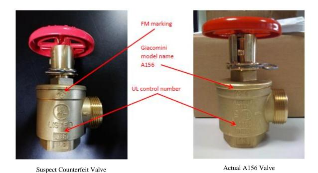
**Figure 1 – Model A156 Valves:** The suspect counterfeit valve has the UL control number identified as "618R". This control number refers to UL File EX2964(Hose Valves) which includes the A55 angle hose valves. The correct control number should be "12HO" which refers to Model A156 and UL File EX3504(Pressure Reducing Devices).
