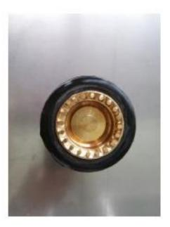
**Figure 3:** Counterfeit A7 1-1/2" Firehose Nozzle (Top View) – The machining of the teeth on the counterfeit nozzles are irregular (randomly squared, trangular, etc).
