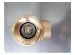
**Figure 6:** Counterfeit A55 1-1/2" Standard Hose Valve (Bottom View) – The nut on the counterfeit valve is made of carbon in comparison to stainless steel which is in accordance with requirements on the actual valve.
