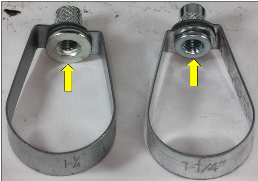
Figure 2. Authentic A-100 (left) with counterfeit AU-100 (right)
