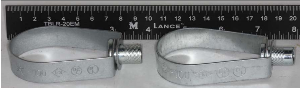
Figure 1. Authentic A-100 (left) with counterfeit AU-100 (right)
