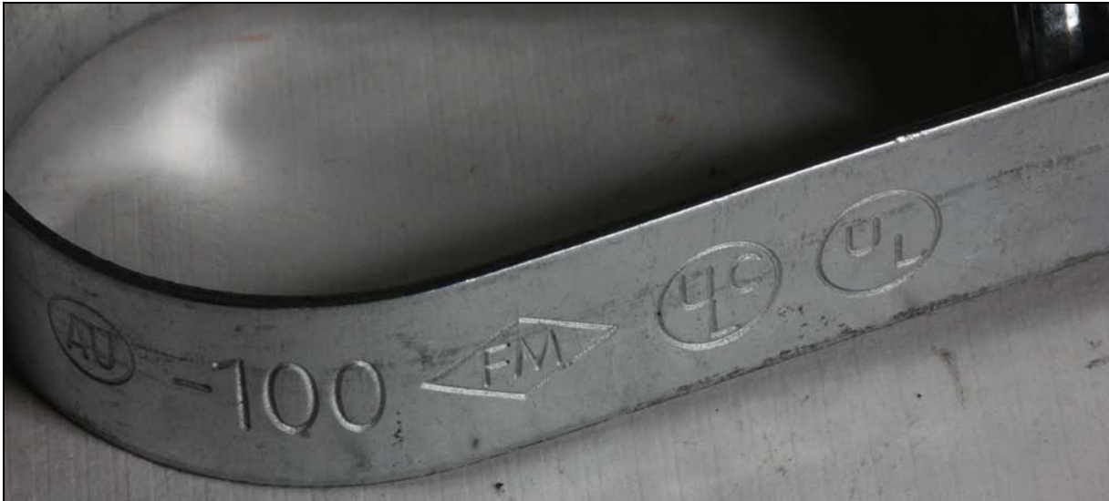
Figure 4. Counterfeit AU-100 pipe hanger markings
