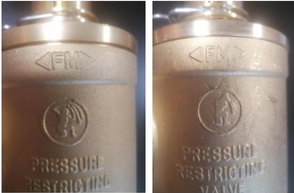
Figure 3. Photographs of a counterfeit A155 pressure restricting valve (left) and an authentic Giacomini SpA, A155 pressure restricting valve (right). There are clear differences between the valve body logo on both pressure restricting valves.
