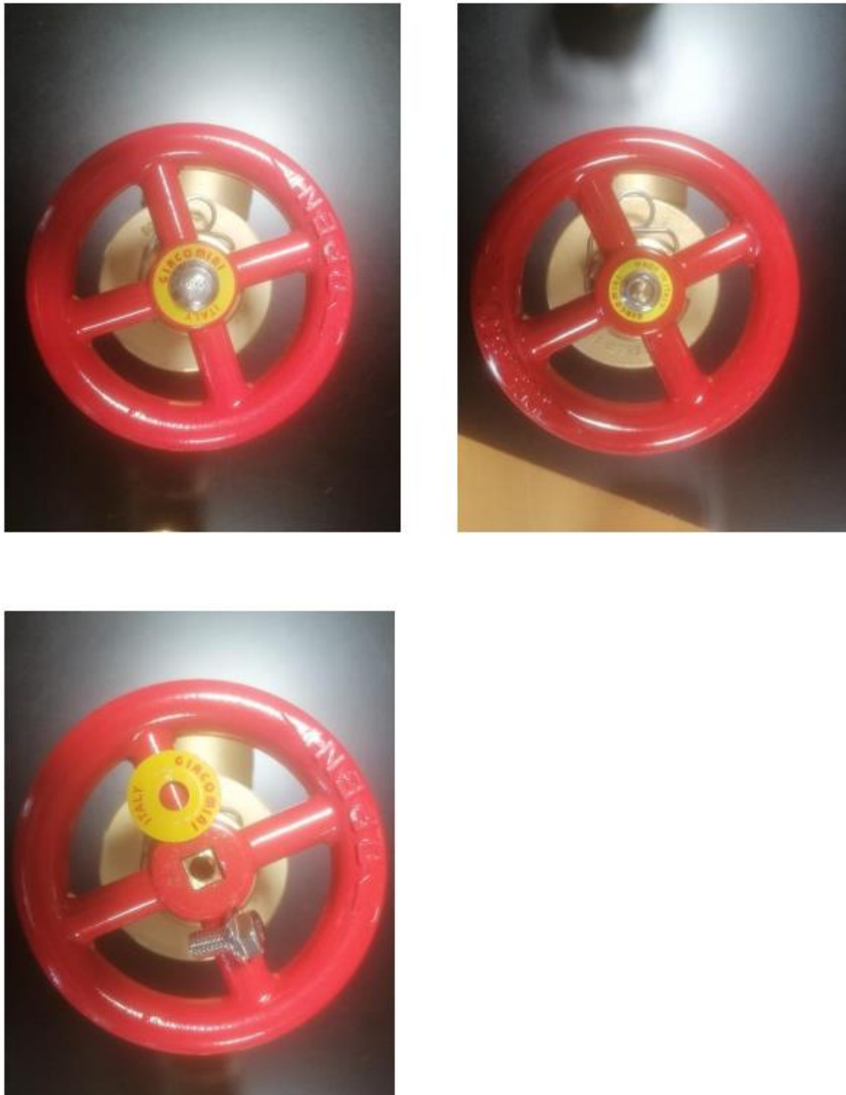
Figure 2. Photographs of a counterfeit A155 pressure restricting valve (left) and an authentic Giacomini SpA, A155 pressure restricting valve (right). The FM Approved A155’s handwheel is secured with a nut (Top) while the suspected counterfeit product’s handwheel is secured with a bolt (Bottom). Also, the suspected counterfeit valve’s yellow ring is a different size and references “ITALY” in comparison with the authentic valve’s yellow ring which clearly states “MADE IN ITALY”.
