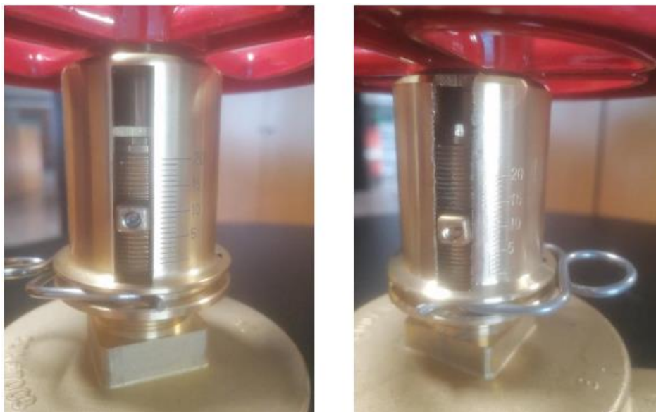
Figure 4. Photographs of a counterfeit A155 pressure restricting valve (left) and an authentic Giacomini SpA, A155 pressure restricting valve (right). The suspected counterfeit product's setting positions are laser etched and are restricted in comparison to the authentic product's settings which are engraved and setting/locking bell range extends to the top.
