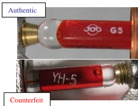
Figure 3. The photographs to the left show enlarged views of the thermal activation elements found in the authentic (top) and counterfeit (bottom) sprinklers. Note the authentic Globe sprinklers utilize the Job model G5 bulb while the counterfeit sprinkler uses a bulb of unknown origin marked with “YH-5.” Also more clearly visible in the photographs are the differences in load screw end profiles that were pointed out in Figure 1.
