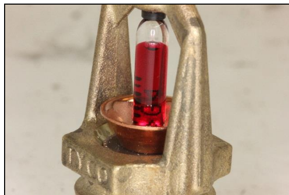
Figure 2. Geissler marking on the glass bulb of an authentic Tyco TY3151 sprinkler. F 900/Rev. 0
