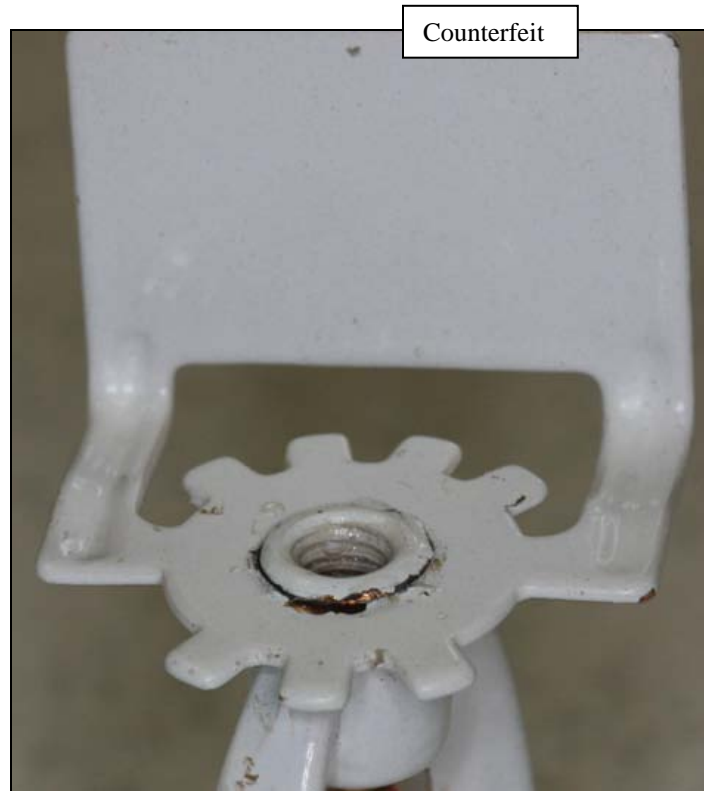
Figure 7 – Deflector design of the counterfeit sprinkler
