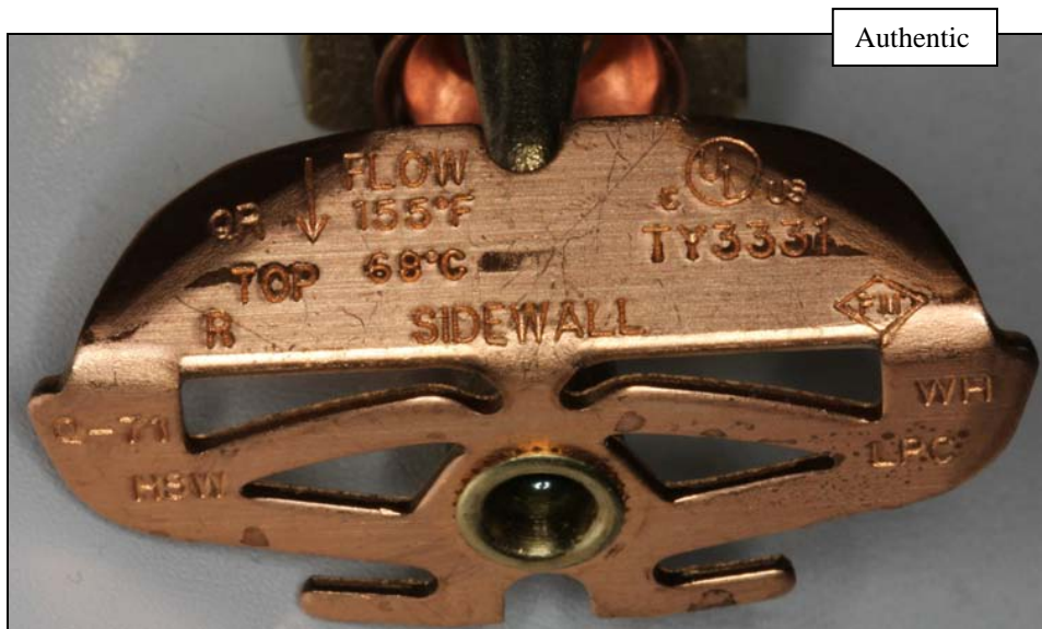
Figure 6 – Deflector of an authentic Tyco TY3351
