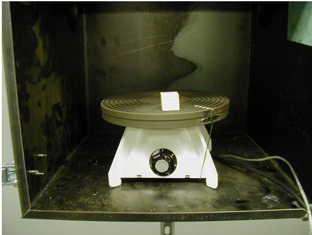
Photo of inside of smoke generation chamber
